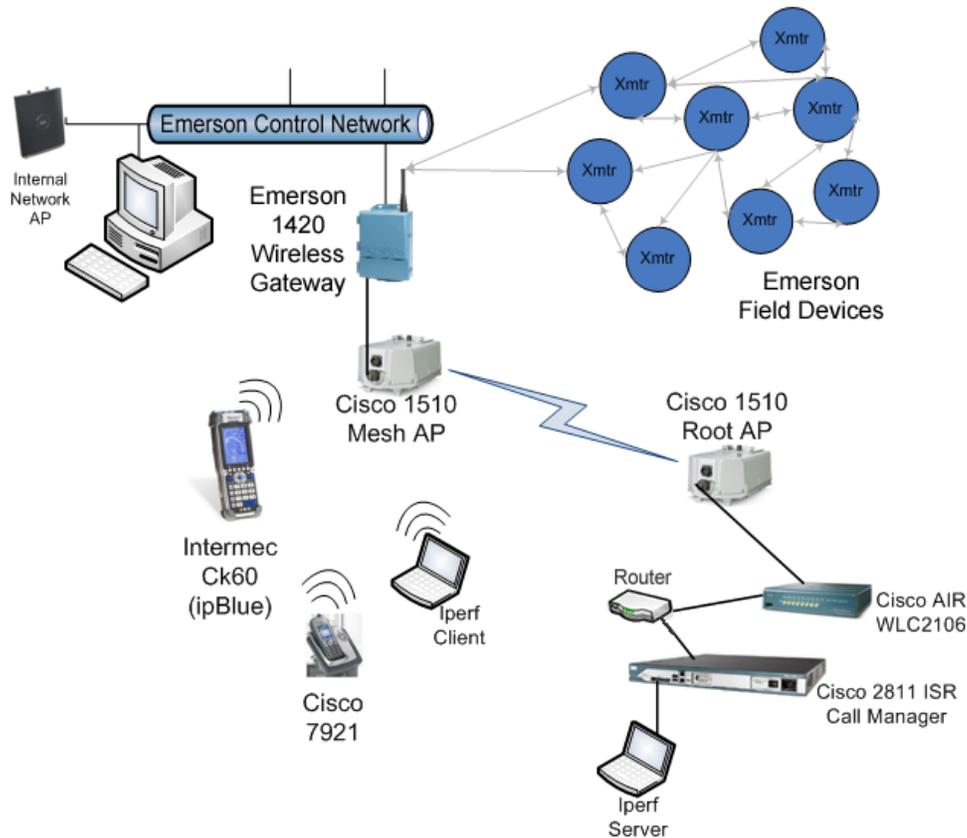
Network performance-analysis tools (an Iperf client and server) were connected to the test access points to provide a load on the Wi-Fi network. To provide voice over Internet protocol (VoIP) traffic, a Cisco 7921 IP phone and an Intermecc CK60 mobile worker platform with a voice application were used.
